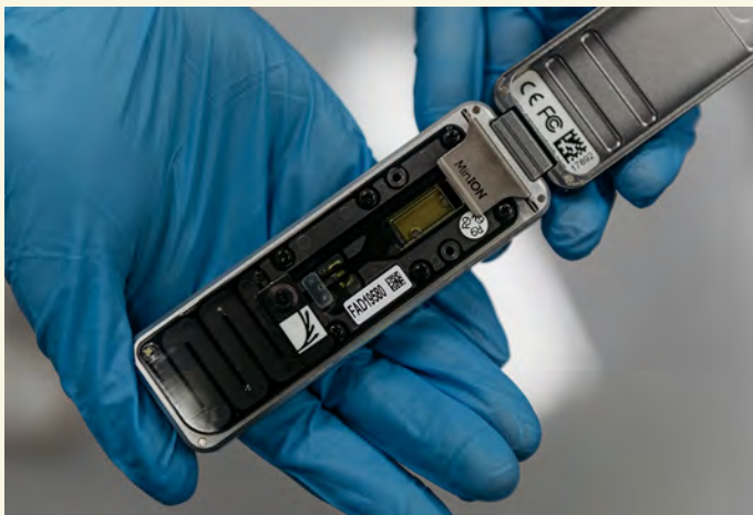
A technician holds an Oxford Nanopore Technologies Ltd. device for DNA and RNA sequencing.
